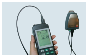
Inspection of transmitters with 4 to 20 mA interface
