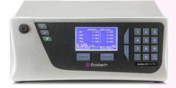
The Serinus® 44 analyser delivers precise and reliable performance at excellent value. It uses proven chemiluminescence technology and an external thermal catalytic converter to measure NO, NO<sub>2</sub>, NO<sub>x</sub> and NH<sub>3</sub> in ambient air (LDL < 0.4 ppb, range 0 to 20 ppm).
