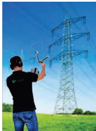
Checking high-voltage overhead lines for corona discharge
