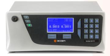
The Serinus® Cal 300 includes an in-built ozone generator and internal zero-air source, as well as a compact reference photometer, providing precise feedback control for accurate ozone generation and measurement in the one unit.
