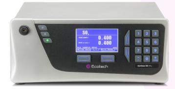
The Serinus® 50 sulfur dioxide (SO<sub>2</sub>) analyser delivers precise and reliable performance at excellent value. It uses proven pulsed UV fluorescent radiation technology to measure SO<sub>2</sub> in ambient air (LDL < 0.3 ppb, range 0 to 20 ppm).
