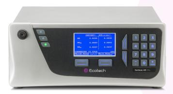
The Serinus<sup>®</sup> 40 Oxides of Nitrogen (NO<sub>x</sub>) analyser delivers precise and reliable performance at excellent value. It uses proven chemiluminescence technology to measure NO, NO<sub>2</sub> and NO<sub>x</sub> in ambient air (LDL < 0.4 ppb, range 0 to 20 ppm).
