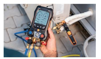
Refrigeration system adjustment made easy: through wireless interaction of our testo 557s, 550s and 550i manifolds with the testo Smart Probes for measuring pressure, temperature and humidity and our testo App.
