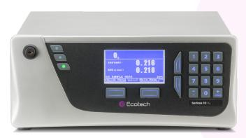
The Serinus<sup>®</sup> 10 Ozone ( $O_3$ ) analyser delivers precise and reliable performance at excellent value. It uses proven nondispersive ultraviolet (UV) absorption technology to measure  $O_3$  in ambient air (LDL < 0.5 ppb, range 0 to 20 ppm).
